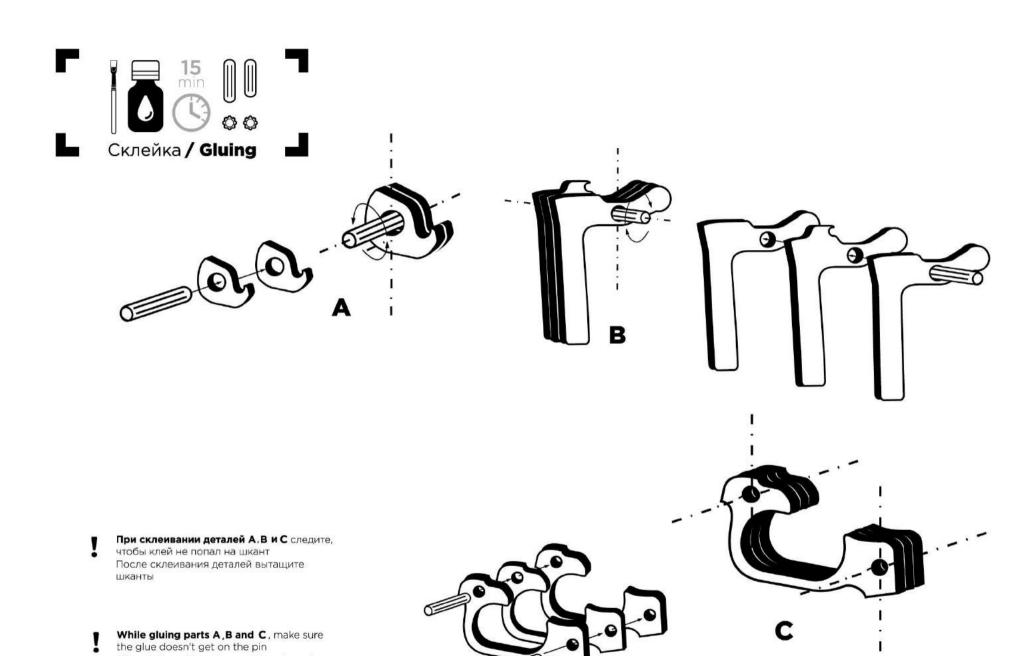
After drying of the glue, pull the pins out
